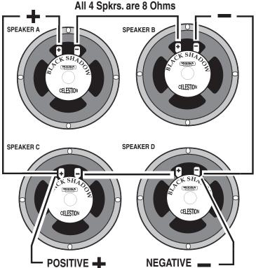
Simply connect the Positive side of Speaker A to the Positive side of Speaker C.
